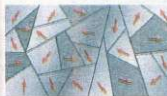
Fig 17.16 Magnetic domains within an unmagnetized ferromagnet.
