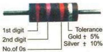
Resistor Colour Code
