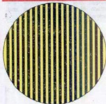
Interference fringes in the Michelson interferometer.
